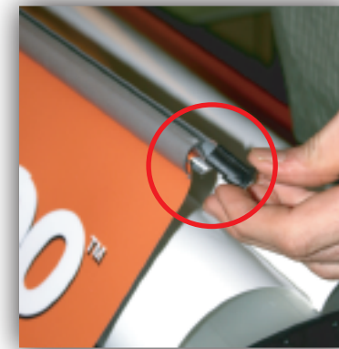
5. REMOVE CAP FROM TOP BAR, AND SLIDE OFF TOP BAR.
