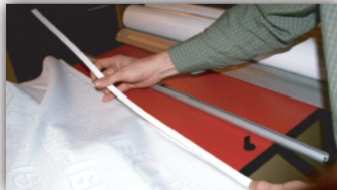
8. PLACE PVC STRIP ON THE TOP OF THE NEW GRAPHIC.
