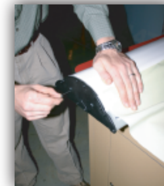
17. FIRMLY HOLD GRAPHIC WHILE RELEASING THE LOCK PIN.
