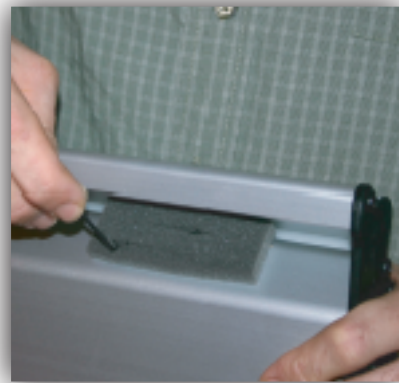
1. REMOVE LOCKING PIN FROM UNDER UNIT.
