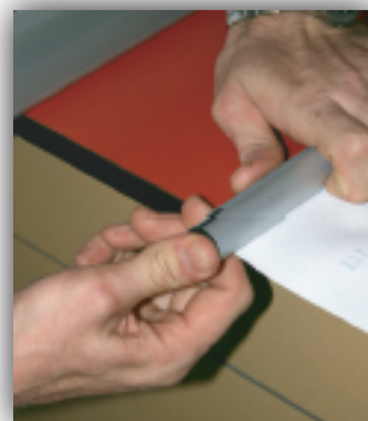
13. CAP ENDS OF THE TOP BAR.
